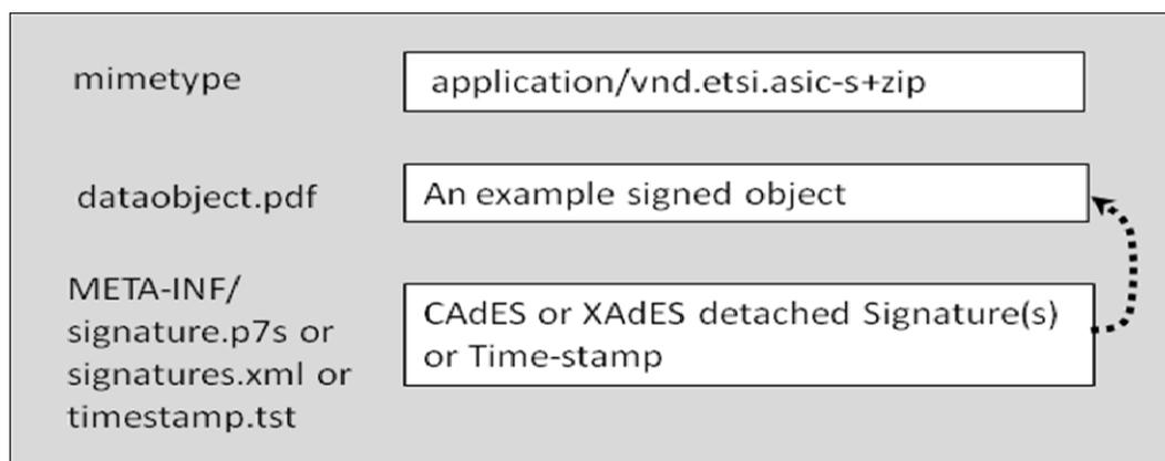
Figure 1: ASiC-S structure applied to a plain data object
