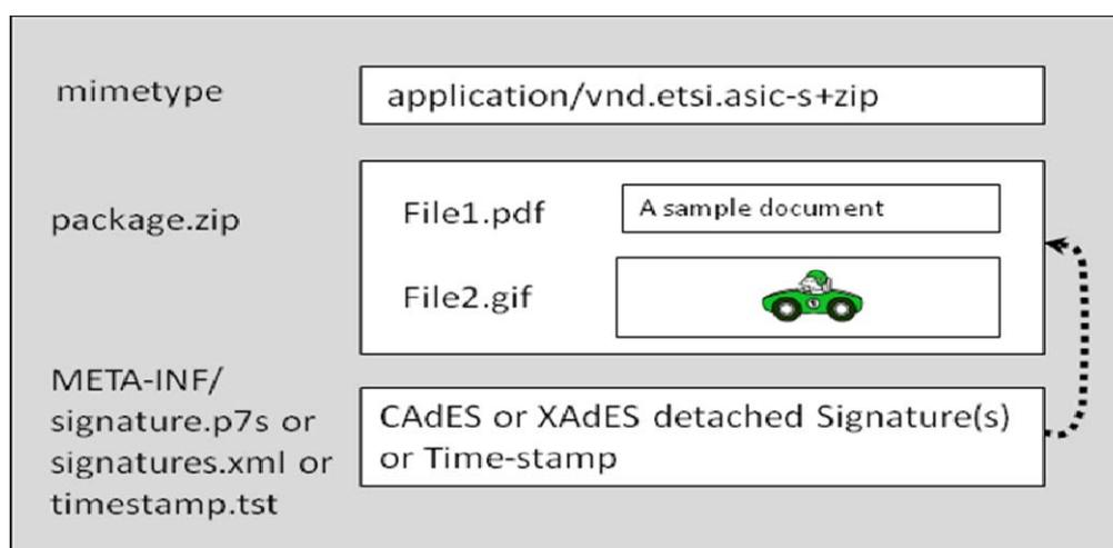
Figure 2: ASiC-S structure applied to a nested container
